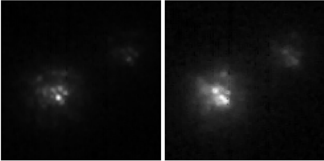
Figure 6: Scientific images (11 mas/px, 1.6 \mu\text{m} , 2-minute long exposure, magnitude 12.8) in closed-loop with the LQG (left, 1:30am, r_0 at 500 nm = 17 cm) and the integrator (right, 1:15am, r_0 at 500 nm = 18 cm).
