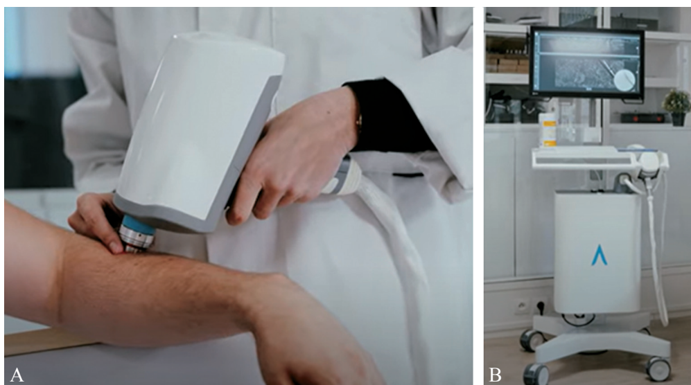
Figure 7.—A) DeepLive™ LC-OCT probe used on a patient; B) full deepLive™ system.
