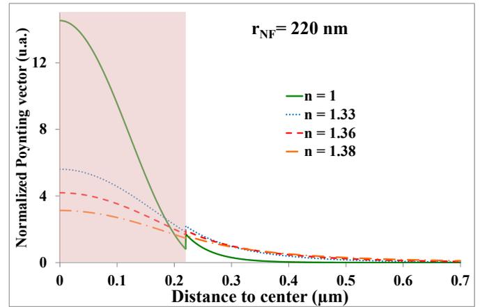
Fig. 3. Normalized Poynting vector  $S_z$  profile for a nanofiber radius of 220 nm for 4 different refractive indexes of the surrounding medium. The colored box shows the limit between the nanofiber and the surrounding medium.
