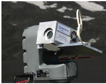
Fig. 4. SIBI (12 cm × 12 cm × 20 cm cube with logos) installed on a rotation stage for gas detection in Etna plume.
