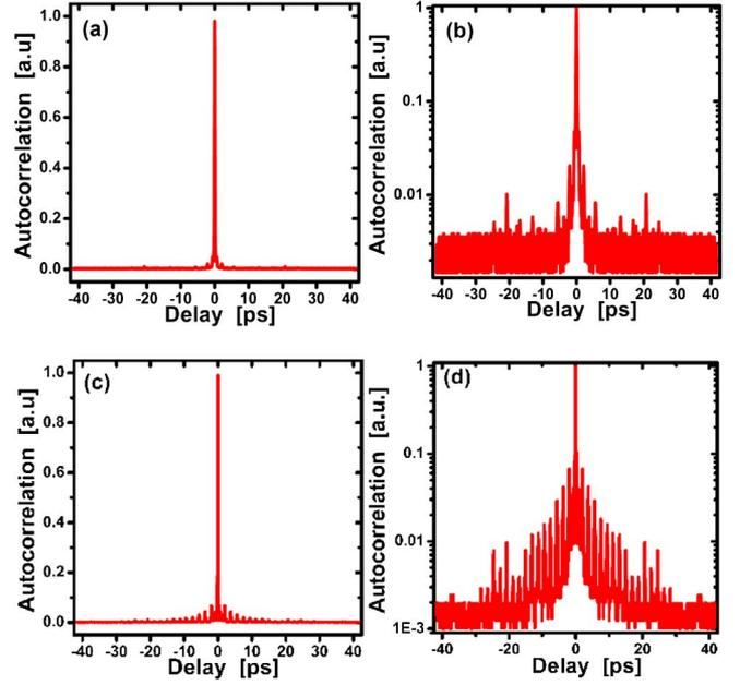
Fig. 4. (a) Long-range autocorrelation in linear scale after compression for 32 replicas at 0.25  $\mu\text{J}$  per replica and (b) corresponding logarithmic scale autocorrelation. (c) and (d) Linear scale logarithmic scale autocorrelation for 32 replicas and 7.5  $\mu\text{J}$  after compression.
