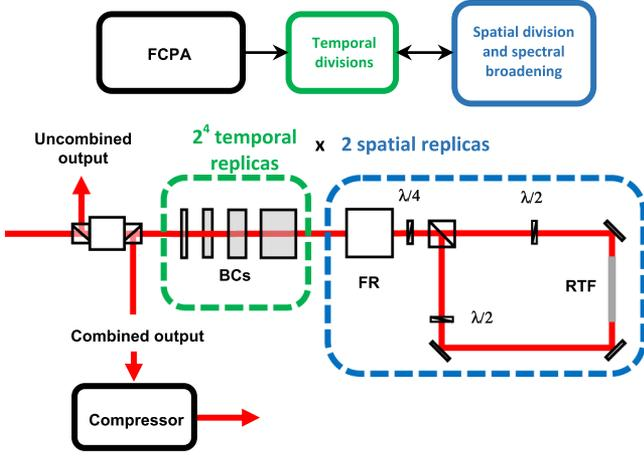
Fig. 1. Experimental spatio-temporal 30 cm × 60 cm postcompression setup. BCs, birefringent crystals; FR, Faraday rotator; RTF, rod-type fiber.
