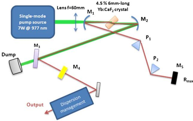
Fig. 1. Experimental setup of the KLM Yb:CaF<sub>2</sub> oscillator.
