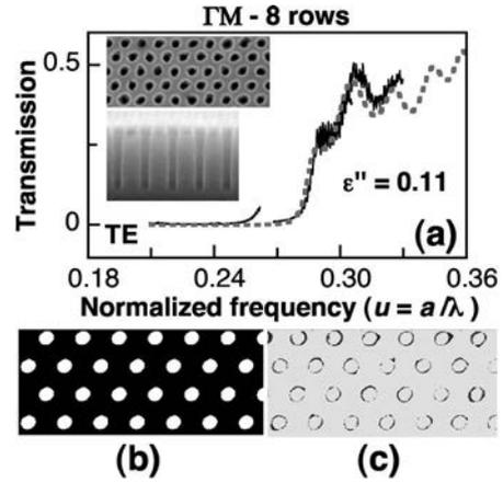
Fig. 2. (a) Measured (solid curves) and calculated (gray dotted curves)  $\Gamma\text{M}$  transmission spectra through eight-row-thick disordered PhC slabs for TE polarization: the value of the loss parameter  $\epsilon''$  is reported; the inset shows the top and edge SEM micrographs. (b) Periodic and (c) disordered components of the top SEM image.
