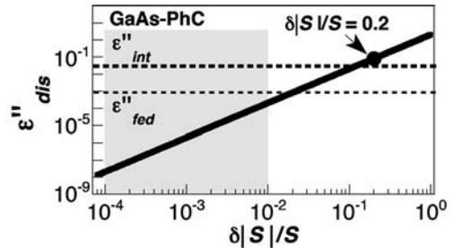
Fig. 3. Disorder-induced losses ( $\epsilon''_{\text{dis}}$ ) as a function of the disorder parameter  $\delta|S|/S$  for GaAs-based PhCs. Circle: the disordered PhC shown in Fig. 2. Dotted lines and gray region:  $\epsilon''_{\text{int}}/\epsilon''_{\text{fed}}$  and  $\delta|S|/S$  values, respectively, for the present fabrication techniques of GaAs-based PhCs.
