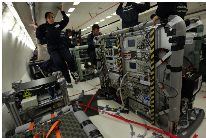
Fig. 2. Experimental apparatus in the plane. The science chamber is protected by a magnetic shield (orange straps, in the front). Behind the science chamber is the rack containing the electrical power supplies and the free-space laser. The bigger unit, on the right, holds the telecom laser source, the 6.8 GHz frequency reference, all the control electronics and the computer.
