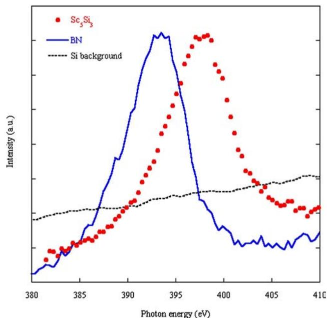
FIG. 2. (Color online)  $N K\alpha$  and  $Sc L\alpha$  emission bands from BN (solid line) and  $Sc_5Si_3$  (dots), superimposed to the background of the  $N K$  domain recorded with a Si target (dotted line).
